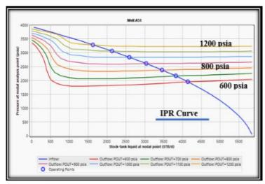
Fig (11) Well Head Pressure Effect on The Flow Rate in well A51
