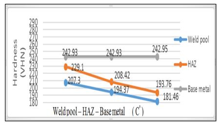
Figure 6: Micro hardness along weld pool, HAZ and base metal at different heat input.
