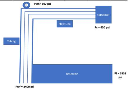
Figure (13) Summary of Nodal Analysis of Pressure Nodes for Well A51
