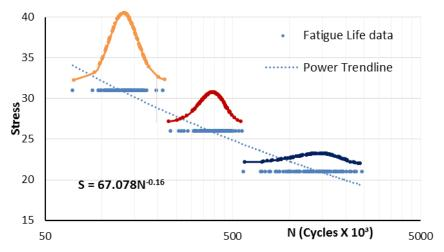
Figure 2. S-N-P curve shows probabilistic nature of fatigue failures at three stress levels.
