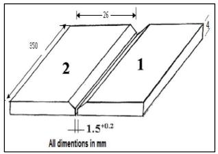
Figure 1: Preparation of the slides for welding process.
