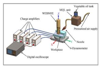
Fig (5) WEBNHE Engaged in End-milling under MQL Cooling
