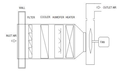
Figure 2. Central Air conditioning unit
