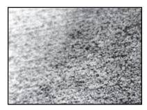
Figure 7: Optical micrograph of TIG welding at low heat input (100x).
