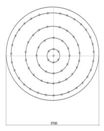
Fig 5. Distribution of anodes at the bottom of tank
