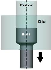
Fig.3. Forward extrusion process
