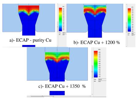
Fig.10.Flow stress simulation diagram when using 9 mm extrusion channel for three types of materials
