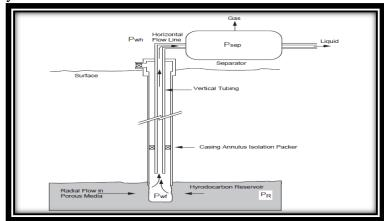
Figure (1) Flow Path and Pressure Nodes from Reservoir to the Separator.
