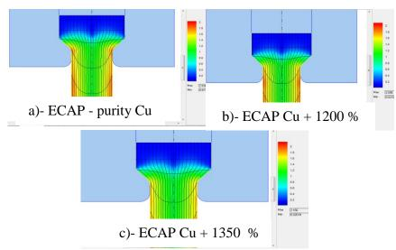
Fig. 12.Effective strain simulation diagram when using 3 mm extrusion channel for three types of materials
