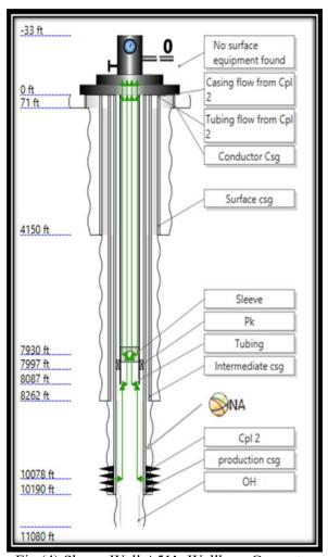
Fig (4) Shows Well A51's Wellbore Geometry
