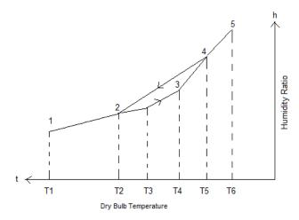
Figure 3. Operation system on the Psychrometric chart
