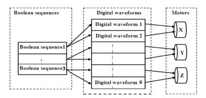
Figure 14: Digital wave form generation
