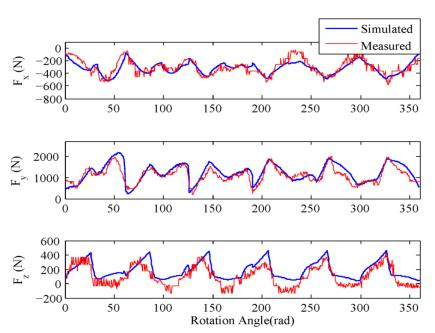
Fig. 6. Measured and predicted (simulated) cutting force components in the end-milling of Inconel 718 using WEBNHE under EM and MQL cooling strategies, at 93 rpm
