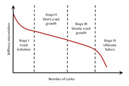
Figure 1. Stages of crack nucleation and growth
