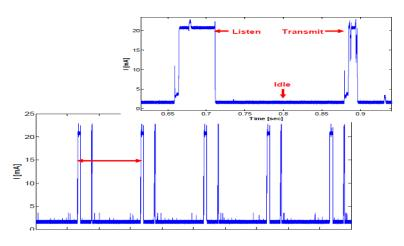
Figure 7. Actis current consumption during 5 seconds of operation. Red arrow marks one super frame cycle.
