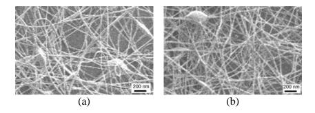
Figure 4. SEM micrographs of PET nanofibers using 0.01 ml/min, flow rate and (a) 0.21 mm (b) 0.26 mm ID of needle.
