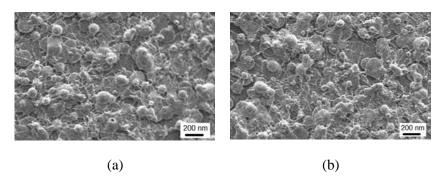
Figure 2. SEM micrographs of PET nanofibers using 0.05 ml/min, flow rate and (a) 0.21 mm (b) 0.26 mm ID of needle
