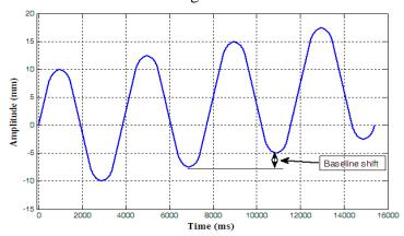
Figure 6: Generate signal with the baseline shift
