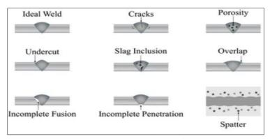
Fig. 4 Welding Defects
