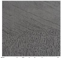
Figure 4: Optical micrographs of medium heat input (100x).
