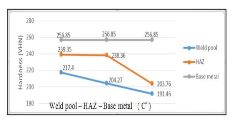
Figure 10: Micro hardness along weld pool, HAZ and base metal at different heat input.
