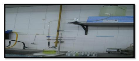
Figure (1) Fixed Bed Adsorber.
