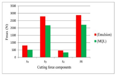
Fig (7) Maximum magnitudes of predicted cutting force components under EM and MQL cooling strategies
