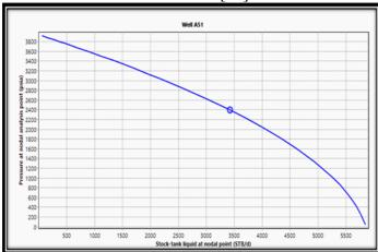
Fig (5) IPR Curve for Well A51
