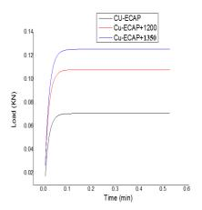
Fig. 7-a. curves of load-time when using 3 mm extrusion channel
