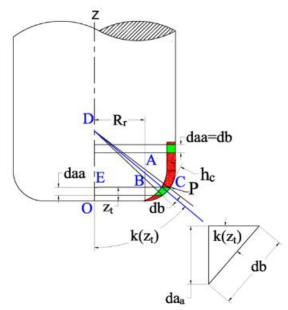
Fig (4) Chip Widths in the Arc and Cylindrical Zones (Sultan and Okafor 2016)
