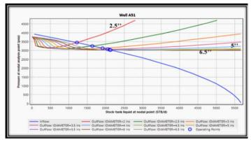
Figure (7) Tubing Size Effect on The Flow Rate for well A51
