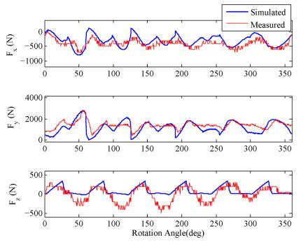
Fig. 6. Measured and predicted (simulated) cutting force components in the end-milling of Inconel 718 using WEBNHE under EM and MQL cooling strategies, at 93 rpm
