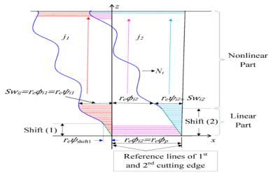
Fig (3) Linear and nonlinear parts of the first two wavy-cutting Edges (Okafor and Sultan 2015)
