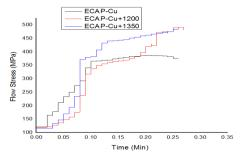
Fig. 11-b. Flow stress curves when using 9 mm extrusion channel
