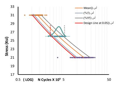
Figure 3. Design curve at 5 % lower bound
