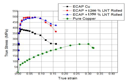
Fig.4. True stress and true strain curves for three Cu samples: as received ECAP Cu, after additional LNT rolling to 1180%, and after LNT rolling to 1340% in addition to pure Cu.
