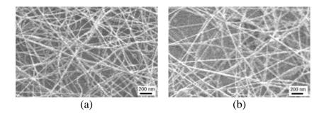
Figure 5. SEM micrographs of PET nanofibers using 0.005 ml/min, flow rate and (a) 0.21 mm (b) 0.26 mm ID of needle
