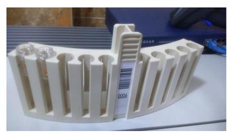
Figure 2. Rack identified by a bar code label
