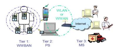
Figure 1. WWBAN integrated into a telemedical system for health monitoring
