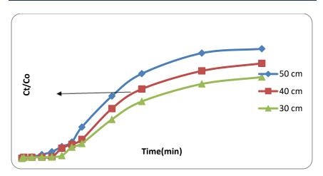
Figure (3) Breakthrough Curves for m-Cresol onto Coconut Shell-GAC for different bed depths, Q =50 ml/min, Co=40 ppm.
