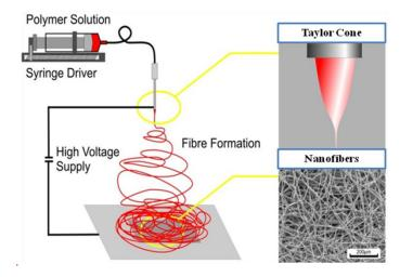
Figure 1. Schematic representation of the applied electrospinning process.
