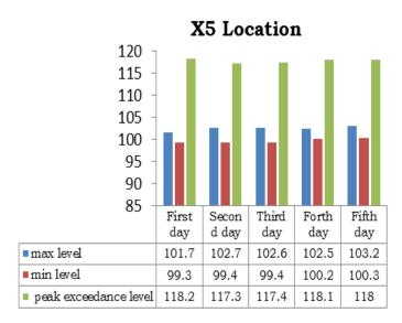
Figure 12. Max, min and peak exceeding level at location X5, STU3
