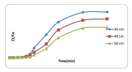
Figure (2) Breakthrough Curves for 4-Nitrophenol onto Coconut Shell-GAC for different bed depths, Q =50 Ml/Min, Co=40ppm.
