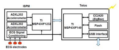
Figure 4. Block diagram of an ActiS sensor node.
