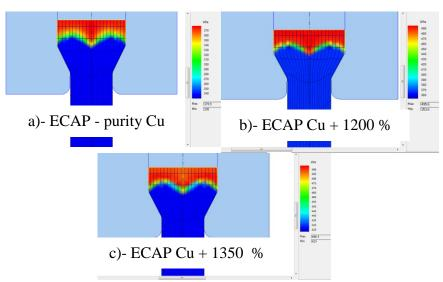
Fig.9.Flow stress simulation diagram when using 6 mm extrusion channel for three types of materials
