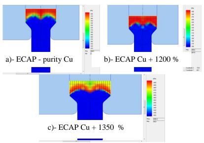
Fig.8.Flow stress simulation diagram when using 3 mm extrusion channel for three types of materials
