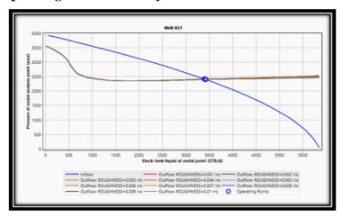
Fig (9) Pipe Roughness Effect on The Flow Rate for well A51
