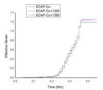
Fig. 15-a. Effective strain curves when using 3 mm extrusion channel
