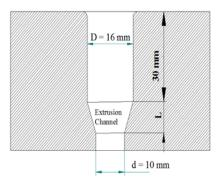
Fig.5. Forward Extrusion Equipment And its dimensions
