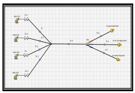
Fig (12) Illustrates the Surface Network of the 4 Wells
