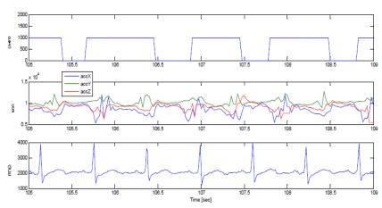
Figure 3. ECG, acceleration, and foot switch data collected by the WWBAN prototype during normal walking.
