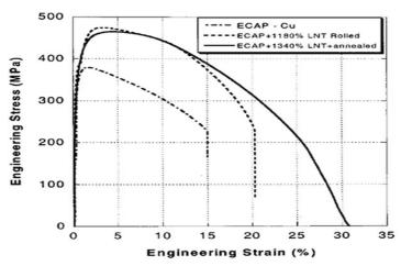
Fig. 2. Tensile engineering stress-strain curves for three Cu samples: as received ECAP Cu, after additional LNT rolling to 1180%, and after LNT rolling to 1340% plus annealing at 100 °C for 2 h [11]
