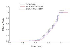
Fig. 15-c. Effective strain curves when using 9 mm extrusion channel
