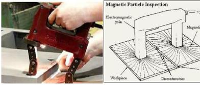
Figs 2 (a) Magnetic particle inspection, (b) Magnetic particle inspection [16].
