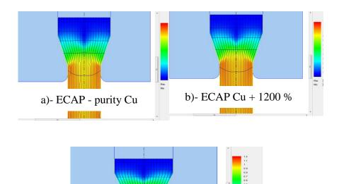
Fig.14. Effective strain simulation diagram when using 9 mm extrusion channel for three types of materials
