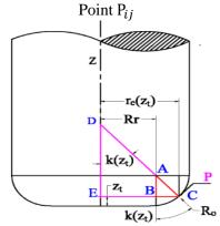
Fig (2-c) Radial Immersion  $r_e(z_t)$  and axial Immersion Angle  $k(z_t)$  of Point  $P_{ij}$  (Okafor and Sultan 2015)
