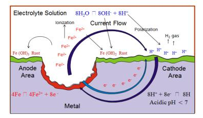
Fig. 2 The electrochemical corrosion[9]
