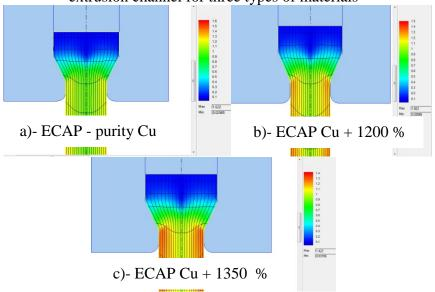
Fig.13. Effective strain simulation diagram when using 6 mm extrusion channel for three types of materials
