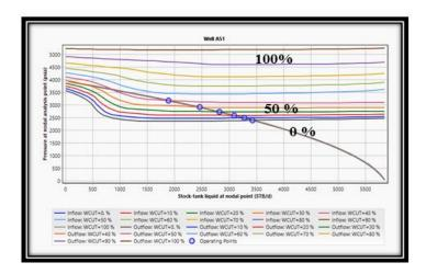
Fig (8) Water Cut Effect on The Flow Rate for well A51
