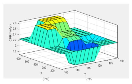
Fig 2: Surface plot of fuzzy logic for CPR
